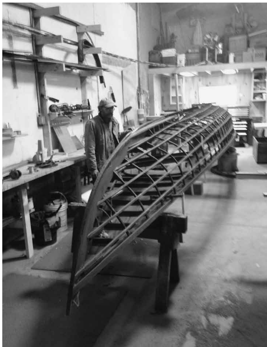
The War Yacht with her nylon skin removed is ready for repairs.
