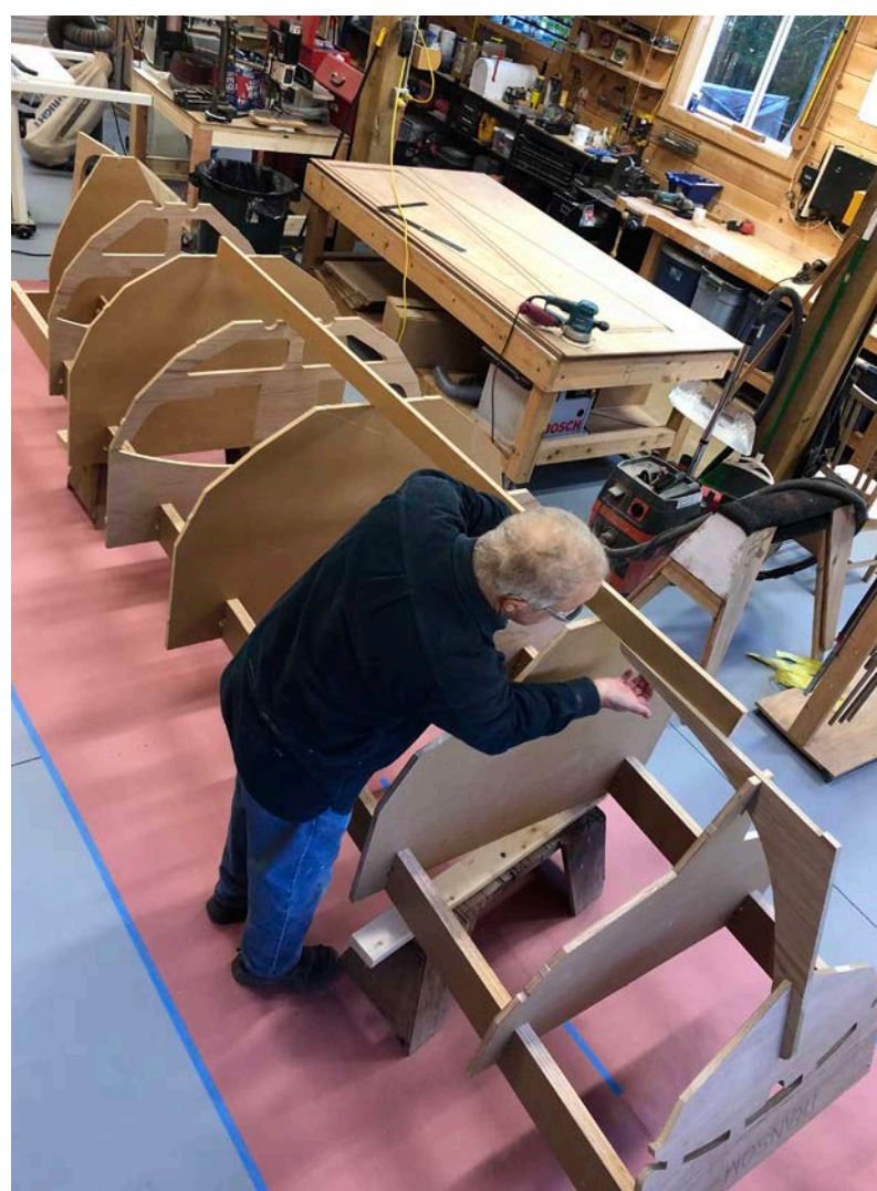
About half an hour later the frame is ready for beveling and planking.
