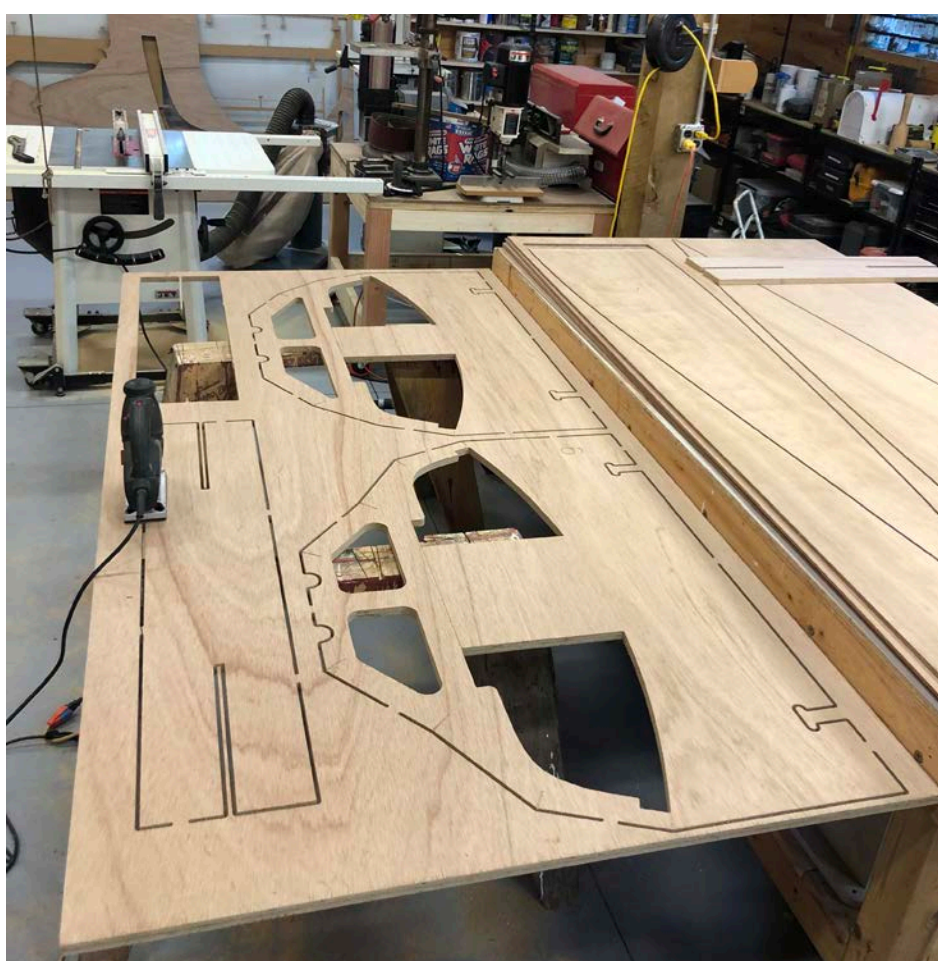
Parts for Stu ’s frame cut by computer and ready to be freed up
